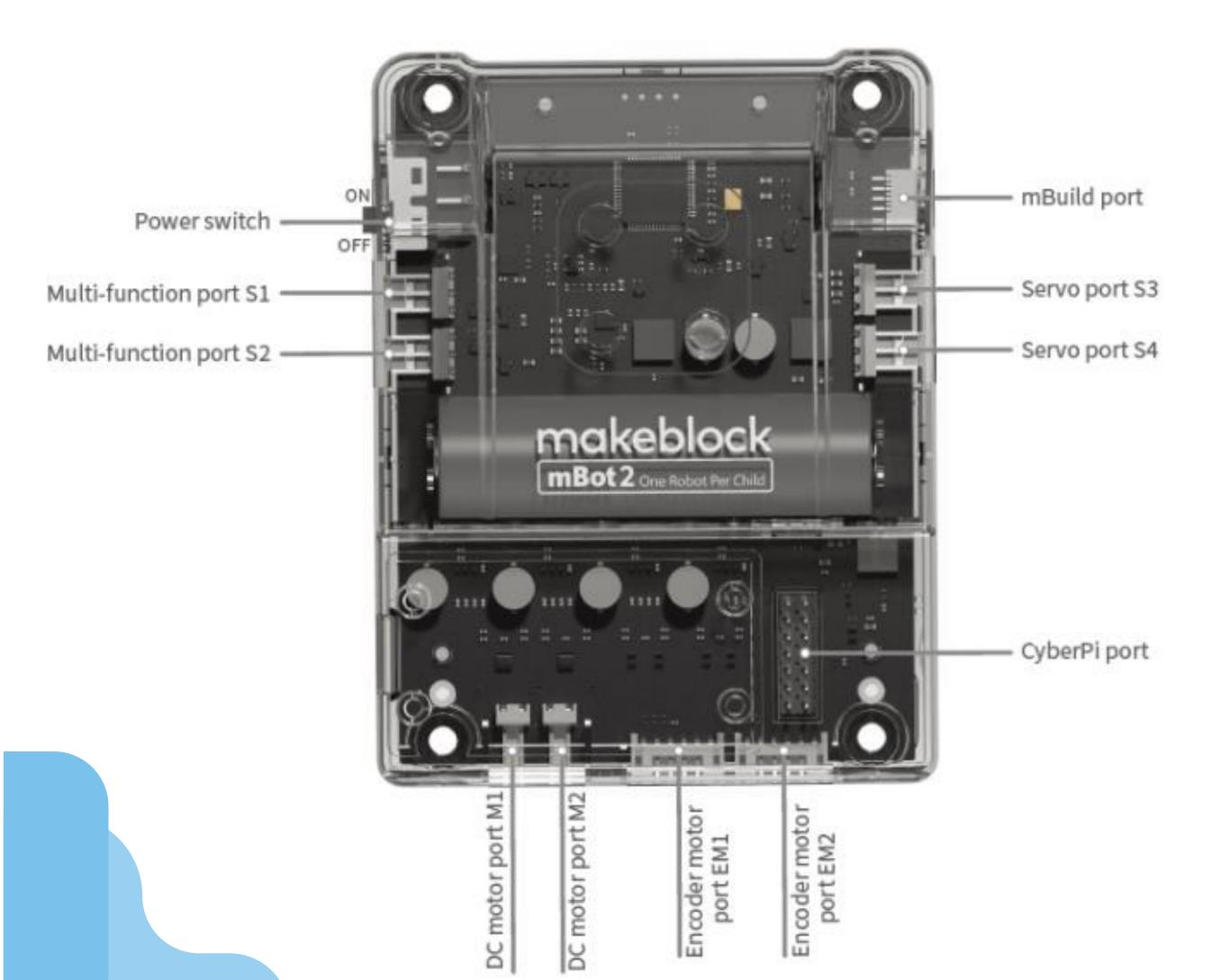
The mBot2 Shield is equipped with a built-in rechargeable lithium-ion battery that can power the CyberPi.
