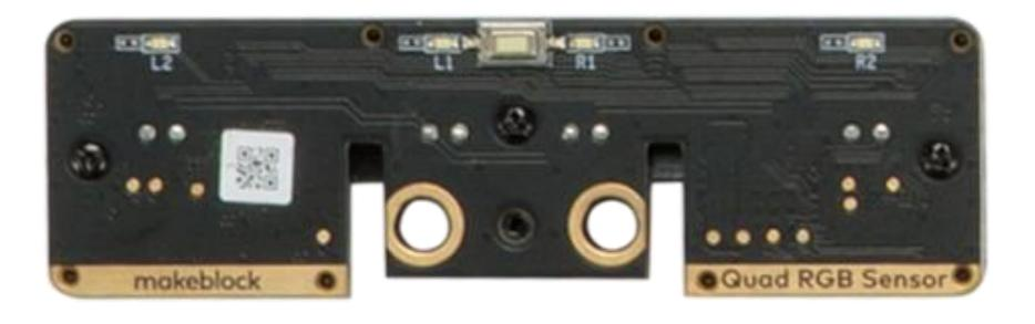
The quad RGB sensor uses visible light as supplemental lights, which significantly reduce ambient light interference. In addition, it provides a color recognition function.
